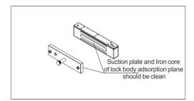
Keep the absorption surface between suction plate and lock clean and tidy, no rust or blot and with good shape. Otherwise, it also will reduce the holding force and no signals will be outputted. The way to solve this problem is to slightly wipe this place with preservative oil.
