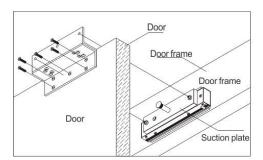
After suction plate and EM lock grip correct, adjust Z shape auxiliary frame, make it top to the door leaf, then locking the screw of Z shape auxiliary frame.
