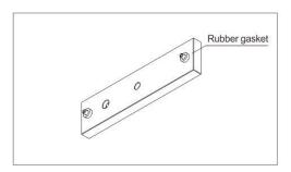
According the picture, set the Rubber washer in the locating pin of Both ends of suction plate.
