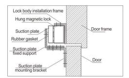
Lastly,fix the Z shape auxiliary frame on the door leaf,closing the door and testing its' suction,the gasket can increase or decrease or tightening the screw,but don't adjust the adsorption gap between suction plate and EM lock,make it completely closed.
