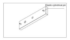
Press-in the accessories' flexible round pin in the toaling hole of suction plate
