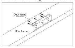
According to L auxiliary frame, paint line in the suitable position of doorframe and fix the L auxiliary frame on the door frame.
