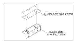
Assembling L-shaped auxiliary frame Z part, the auxiliary frame can be moved
