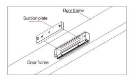
Put the suction plate in the right place of electromagnet part, switch on the power and close the door.
