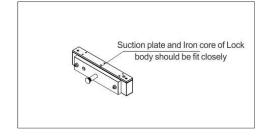
The lock body must be completely aimed at the suction plate. Otherwise, it will lead to reduce the holding force and no reaction from the inner Howard Element. Finally no any signals will be outputted.
