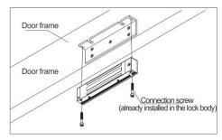
Fix the Electromagnetic lock on L-shaped auxiliary frame with socket head wrench.
