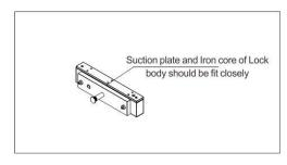
The lock body must be completely aimed at the suction plate. Otherwise, it will lead to reduce the holding force and no reaction from the inner Howard Element. Finally no any signals will be outputted.
