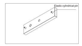
Press the accessories of elastic cylindrical pin into the location hole of suction plate.
