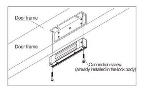
To fix magnetic lock on the L auxiliary frame with the help of allen wrench.
