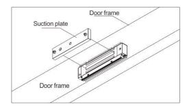
Fix Z auxiliary frame to the door leaf and close the door to test suction. One can increase or decrease gasket or tighten the suction plate screw to make it fully closed instead of adjusting the space between the suction plate and magnetic lock.
