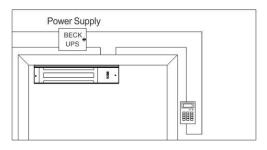
EM lock is fail safe. We suggest you equip the UPS in case of the situation when the power is off to be more safe and secure.
