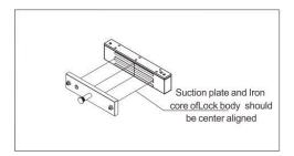
Whatever the installation way you choose, the lock body must be completely aimed at the suction plate. Otherwise, it will greatly reduce the holding force or maybe just a pull can also open the door.
