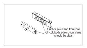
The lock body must be completely aimed at the suction plate. Otherwise, it will lead to reduce the holding force and no reaction from the inner Howard Element. Finally no any signals will be outputted.
