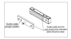
Keep the absorption surface between suction plate and lock clean and tidy, no rust or blot and with good shape. Otherwise, it also will reduce the holding force and no signals will be outputted. The way to solve this problem is to slightly wipe this place with preservative oil.
