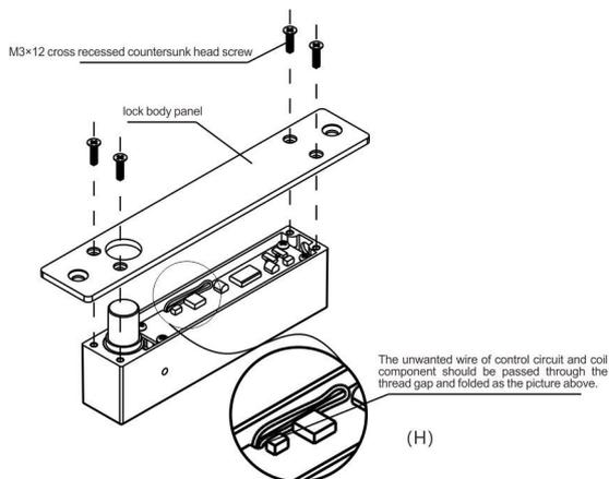
Press the body cover with screw fastened as picture H.
