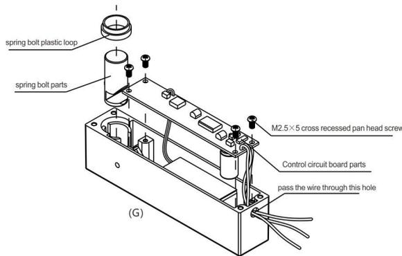
1. Click the spring bolt into the body and spring bolt plastic loop on it as picture G.
