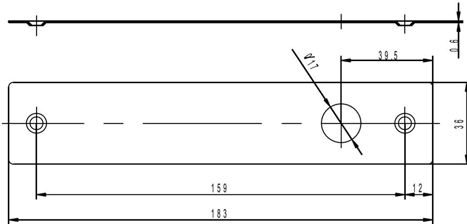
NOTICE: Put the Stainless steel cover board to cover the lock face after installation.
