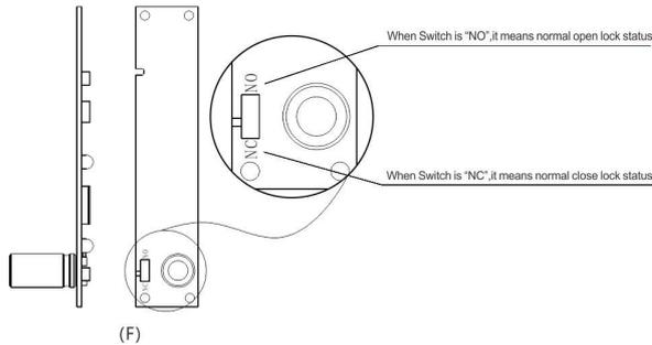
According to the body state, adjust the set switch which is at the back of the control circuit board as picture F.
