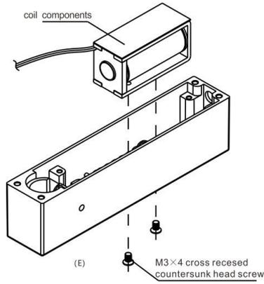
Place the coil components as Picture E, and then fasten the screws.
